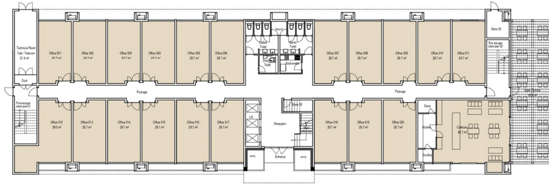
GROUND FLOOR PLAN GROSS AREA (Main Building) = 986 m 2 Entrance = 17.9 m 2 Open Terrace = 83.8 m 2
